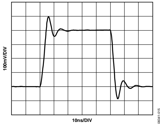
Figure 40. Small Signal Transient Response, G = 12.04 \text{ dB}
