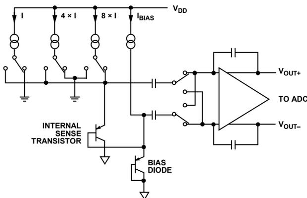
Figure 24. Top-Level Structure of Internal Temperature Sensor
