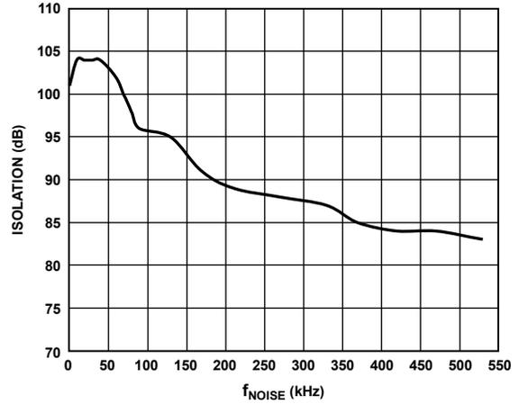
Figure 12. Channel-to-Channel Isolation,  $f_{IN} = 50$  kHz
