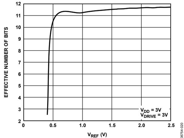
Figure 8. Effective Number of Bits vs.  $V_{REF}$
