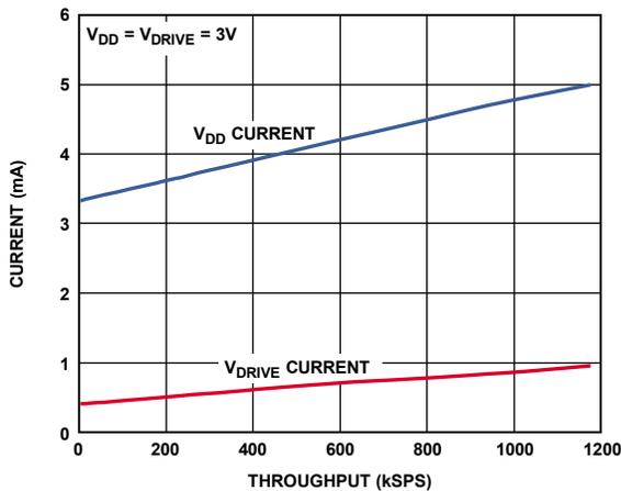
Figure 17. Average Supply Current vs. Throughput Rate
