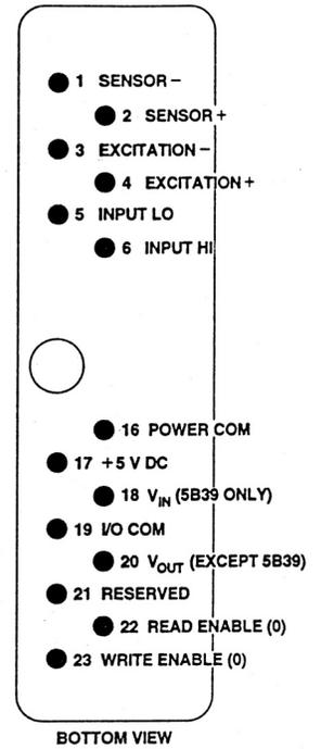
Figure 4 . Model 5B Series Module, with pin-out assignments.
